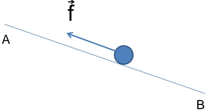
A diagram showing a blue sphere sliding down a blue incline from point A to point B. A blue arrow labeled  $\vec{f}$  points up the incline, indicating the direction of friction. The incline is labeled with points A at the top and B at the bottom.
