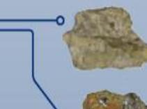
Graphite is used for the anodes of lithium-ion batteries because of its electrical and thermal conductivity.
