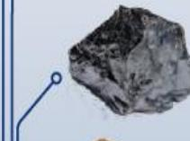
Arsenopyrite is a source of arsenic, which is used in radio frequency and power amplifiers.
