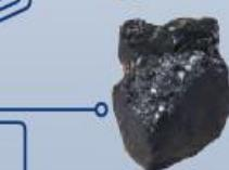
Wolframite is a source of tungsten, which acts as a heat sink and provides the mass for mobile phone vibration.
