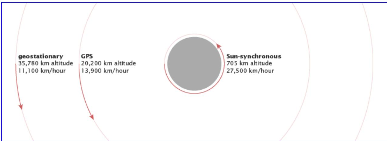
*The higher a satellite's orbit, the slower it moves. Certain orbital altitudes have special properties, like a geosynchronous orbit, in which a satellite travels around the Earth exactly once each day. The length of each red arrow in this diagram represents the distance traveled by a satellite in an hour. View animation. (NASA illustration by Robert Simmon.)*
